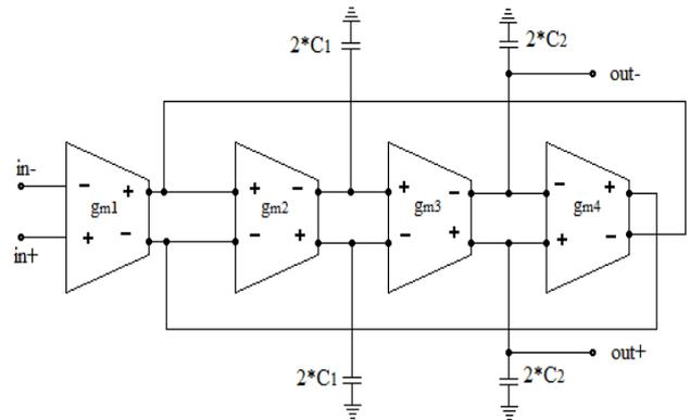
Figure 4: 2<sup>nd</sup> order Gm-C low-pass filter circuits
