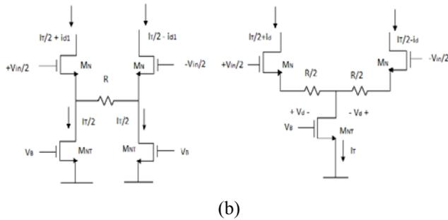
**Figure 1:** differential pairs: a)conventional differential pair; (b) differential pair with degeneration resistance; and (c) differential pair with degeneration resistance and tail current transistor
