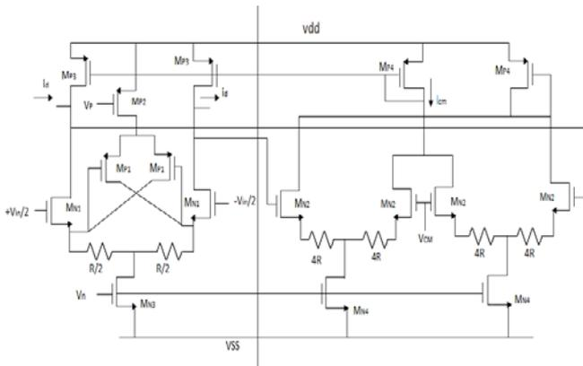
Figure 3: Complete Transconductor with common mode feed-back
