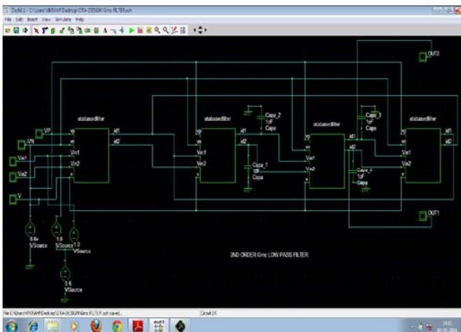
Figure 6: Circuit of 2<sup>nd</sup> order Gm-C filter.
