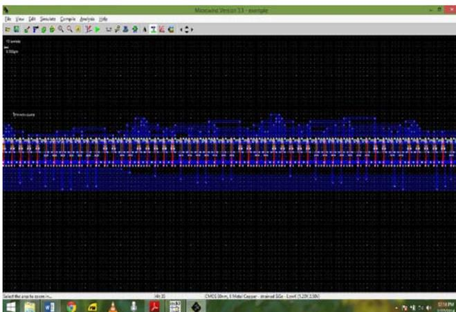
Figure 11: Layout of 2<sup>nd</sup> order Gm-C filter
