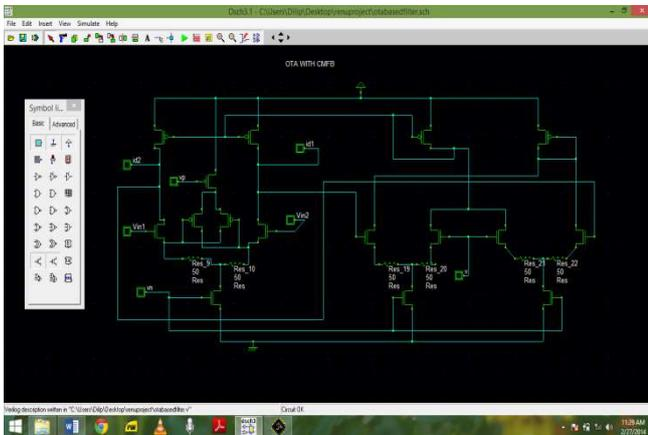
Figure 5: Operational transconductance amplifier (OTA) including common mode feedback (CMFB)
