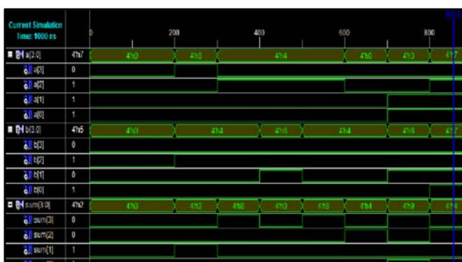
Figure 9: Simulation of proposed BCD Adder
