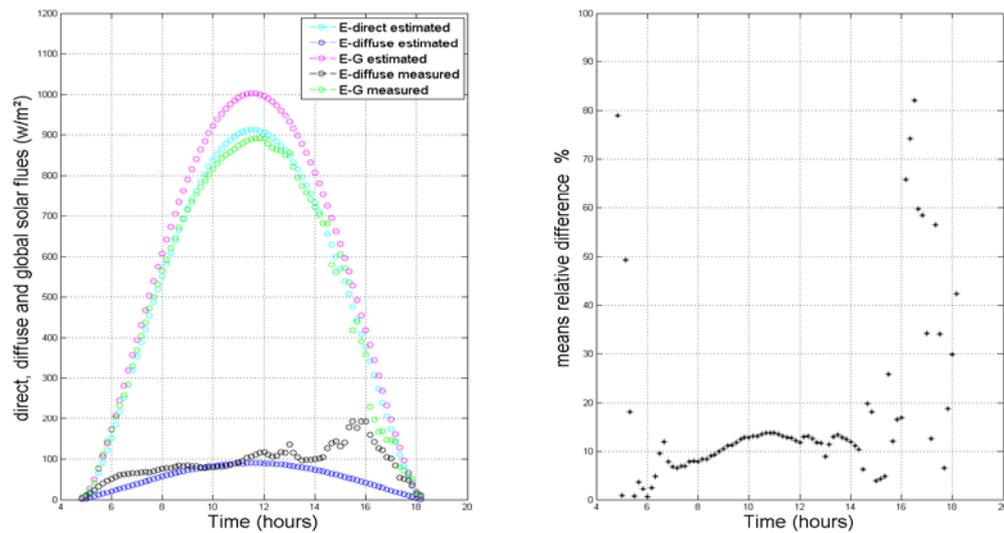
Figure 10 : direct, diffuse and global solarflues & means relative defference for 10 August 2013
