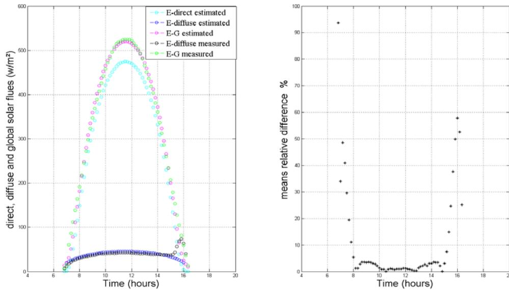
Figure 3 : direct, diffuse and global solar flues & means relative defference for 6 January 2013
