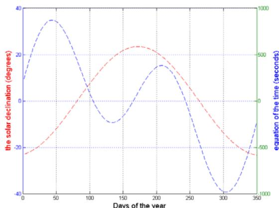
Figure 1: The evolution of the solar declination and equation of the time during the year
