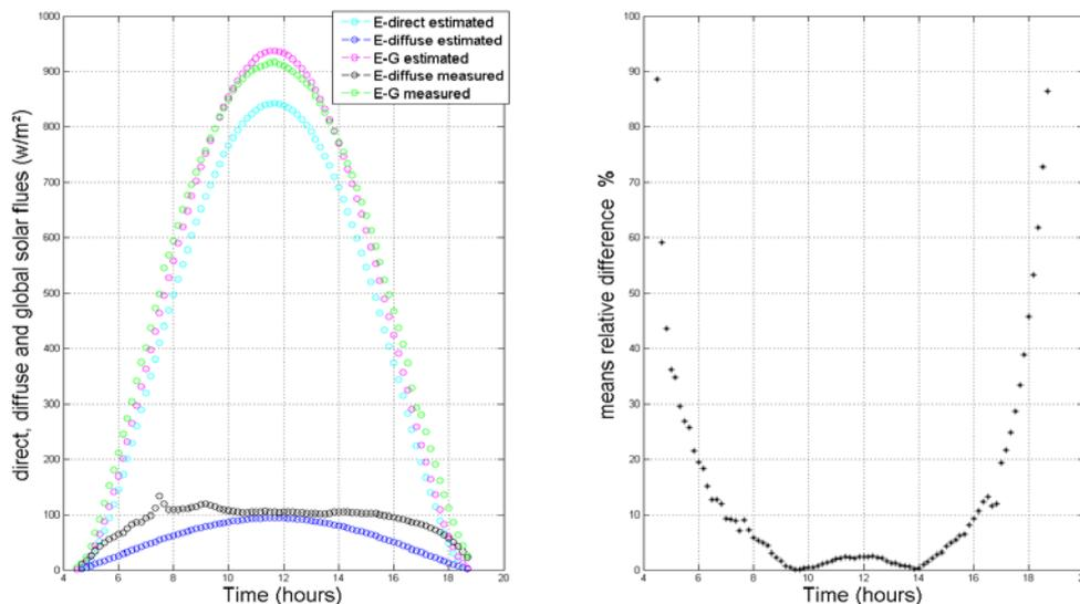
Figure 8 : direct, diffuse and global solar flues & means relative deference for 12 June 2013
