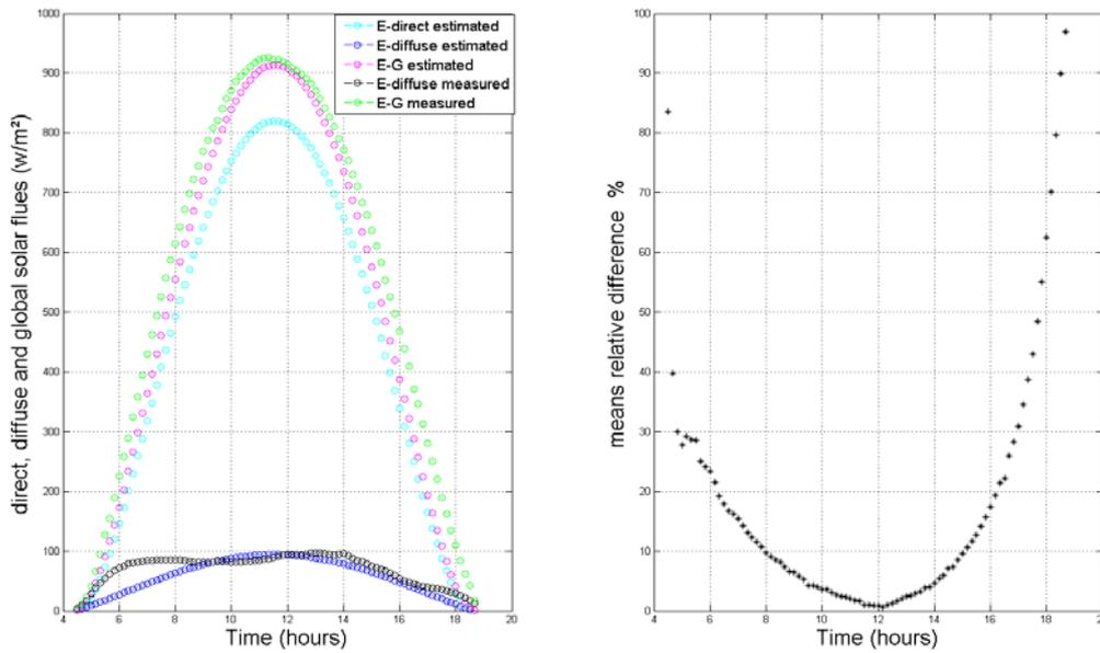
Figure 9 : direct, diffuse and global solar flues & means relative defference for 10 July 2013
