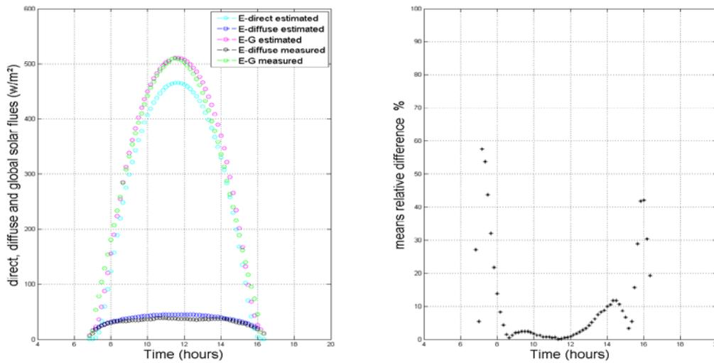
Figure 6 : direct, diffuse and global solar flues & means relative deference for 28 December 2013
