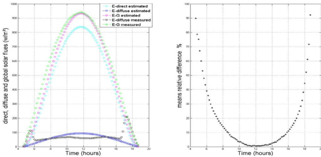
Figure 7 : direct, diffuse and global solar flues & means relative deference for 24 May 2013
