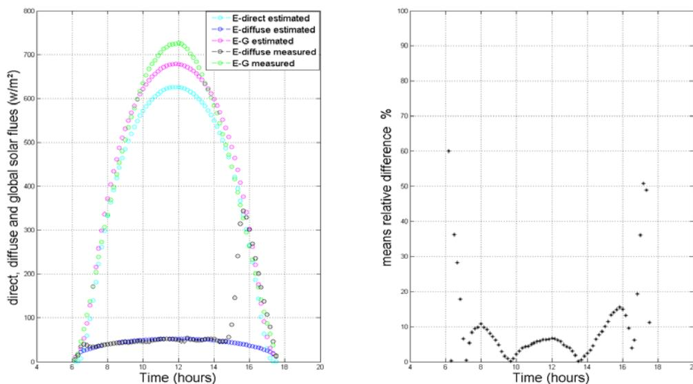
Figure 5 : direct, diffuse and global solar flues & means relative defference for 4 October 2013
