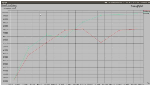
Figure 3.5, Green Color represents Prophet and Red represents Epidemic showing results of throughput.
