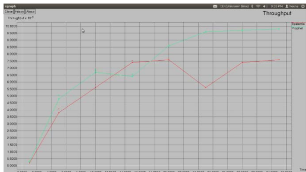
Figure 3.5, Green Color represents Prophet and Red represents Epidemic showing results of throughput.
