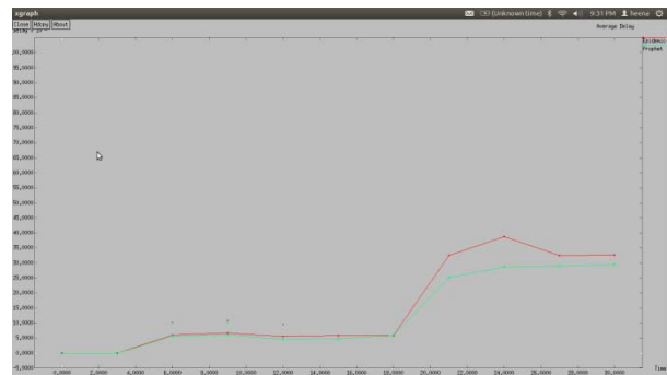
Figure 3.2, Green Color represents Prophet and Red represents Epidemic showing results of Delivery Delay.
