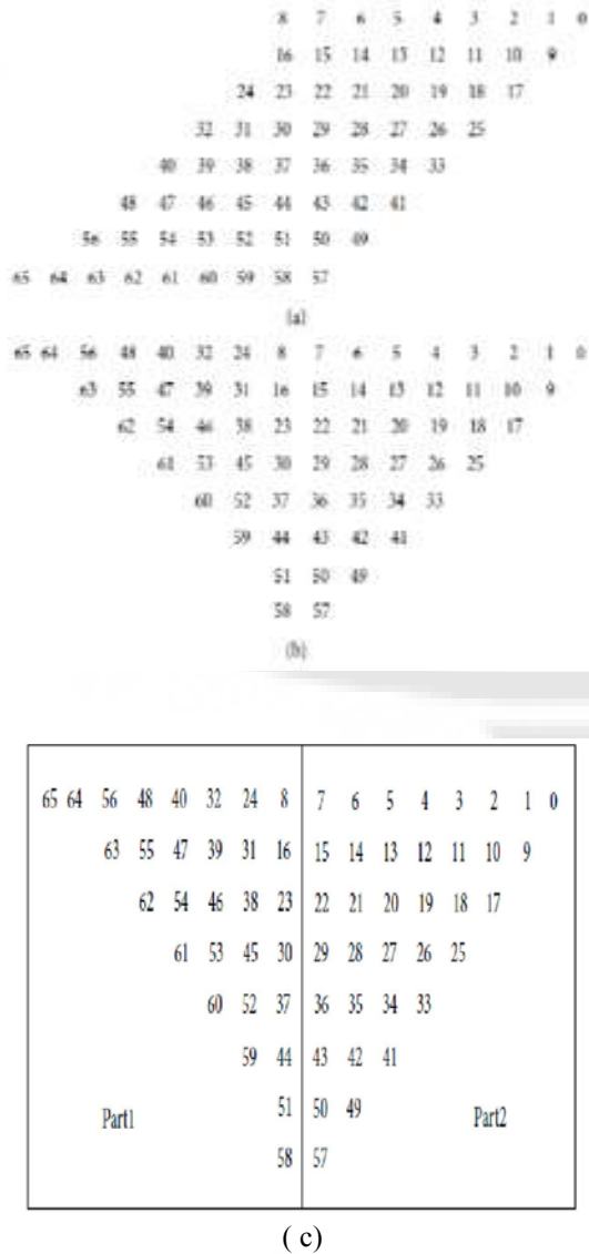
Figure 1: Partitioning the partial products: (a) partial-product array diagram for 8 multiplier, (b) an alternative representation, and (c) partitioned structure of multiplier showing part0 and part1
