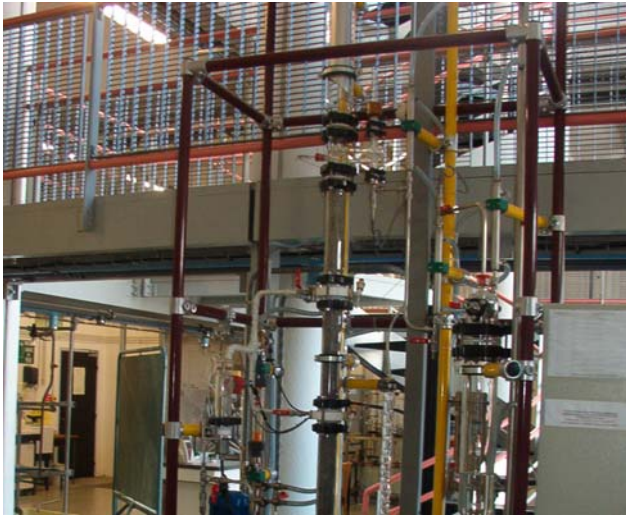
Figure 2: Installation of continuous distillation
