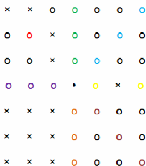
Figure 2: Considered pixels in directional median inpainting, \circ shows a known pixel, \times shows an unknown pixel, color pixels show considered pixel in different directions.
