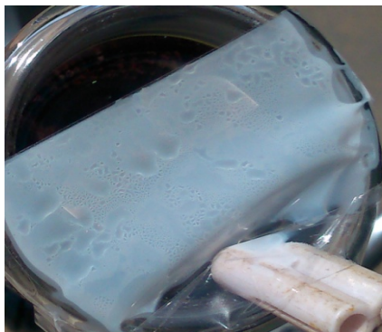
Figure 2: Due to solar heating evaporation starts
