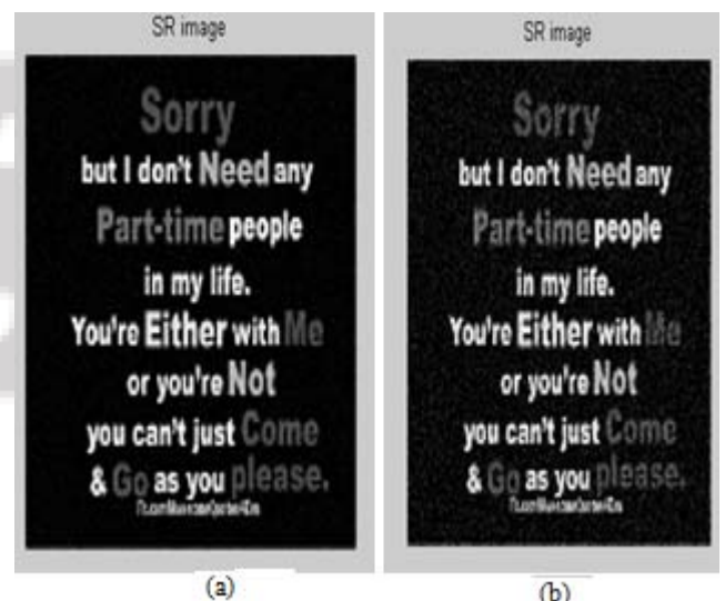
Figure 4: Results of IBP under high noise. Super-resolved image with blur 0.05, 0.066, 0.07, 0.08, (a) with noise=0.1 and (b) with noise=0.2.
