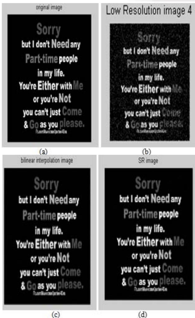
Figure 2: (a) Original HR image, (b) LR image, (c) Bilinearly interpolated image, (d) SR image using IBP
