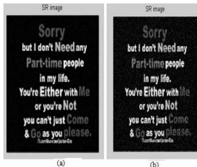
Figure 4: Results of IBP under high noise. Super-resolved image with blur 0.05, 0.066, 0.07, 0.08, (a) with noise=0.1 and (b) with noise=0.2.
