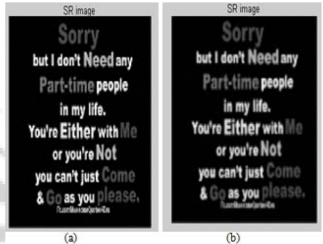
Figure 3: Results of IBP under high blur. Super-resolved image with noise=0.0001 (a) with blur 0.1, 0.2, 0.3, 0.4, and (b) with blur 0.5, 0.6, 0.7, 0.8.
