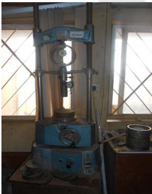
Figure 1: Penetration piston machine used at the Geotechnical and structural Centre, Oshogbo osun state
