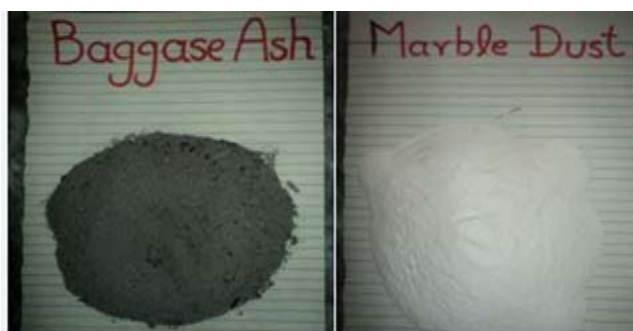
Figure 5: Stabilization material (bagasse ash, marble dust) collected from local factory,
