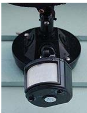
Figure 1: A motion detector attached to an outdoor, automatic light.
