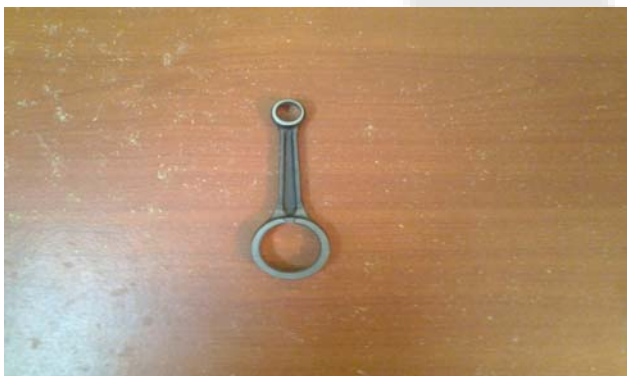
Figure 1: Standard size cast iron connecting rod specimen
