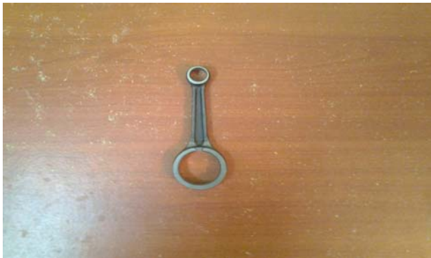
Figure 1: Standard size cast iron connecting rod specimen
