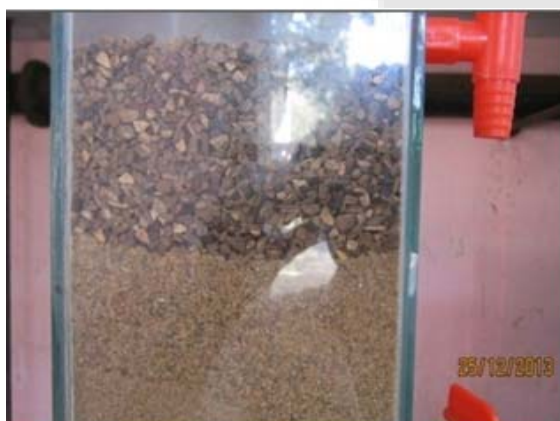
Figure 2: Photograph of capped sand media
