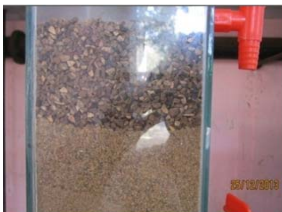
Figure 2: Photograph of capped sand media
