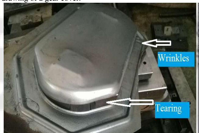
Figure 1: Tearing and wrinkling problem faced during drawing gear cover
