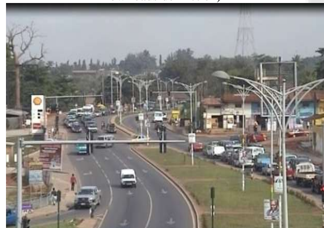
Figure 3: The Asokwa Signalized Intersection (medium roadside friction)
