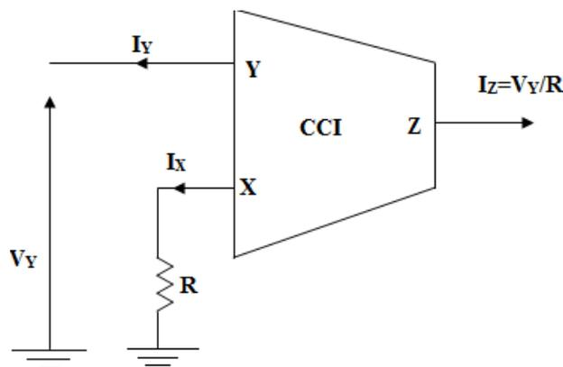
Figure 4: Voltage-to-Current Conversion [6]
