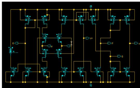
Figure 7: CMOS implementation of the proposed CCII [1]
