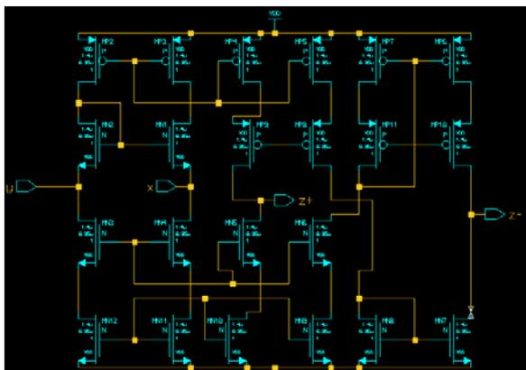
Figure 2: CMOS implementation of the proposed CCI [4]
