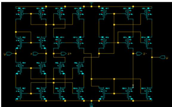
Figure 9: CMOS implementation of the proposed CCIII [4]
