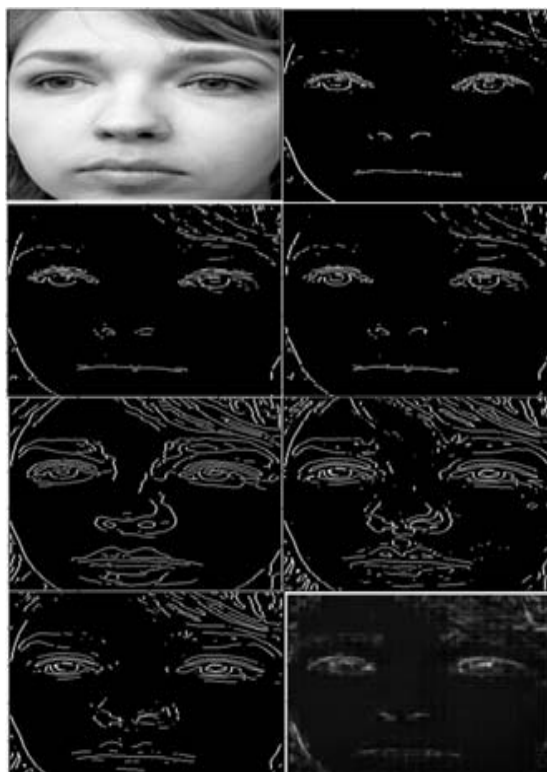
Figure12:-a)Original Image(face.png) b)Robert’s c)Sobel d)Prewitt e)Canny f)Laplacian g)LOG h)Gabor Filter
