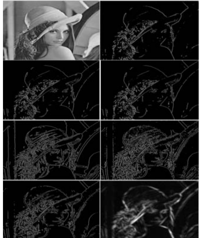
Figure17: a)Original Image(leena.jpg) b)Robert's c)Sobel d)Prewitt e)Canny f)Laplacian g)LOG h)Gabor Filter
