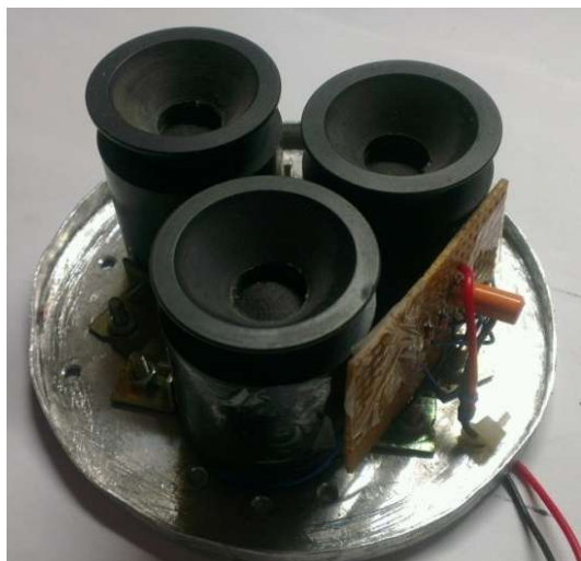
Figure 11: Electromagnetic transducer Mechanism
