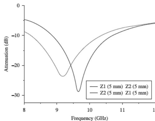
**Figure 8:** Simulations of two-layer RAM's attenuation of electromagnetic radiation as a function of frequency, thickness and stacking order of the absorbing materials. Z1, RAM produce with L9000 silicone rubber; Z2, RAM produce with RTC6300 silicone rubber: both layers are 5mm thick [2]
