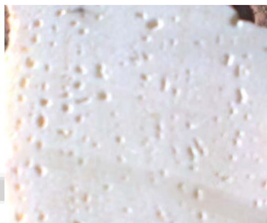
Figure 2: A photograph of a hand specimen, showing vesicular texture in the white band
