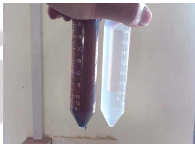
Figure 5: Before and After Degradation with Bimetallic Catalyst (Congo Red)
