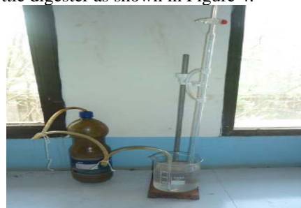
Figure 4: Measurement of biogas volume by water displacement technique.
