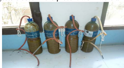
Figure 1: 1.8 L plastic bottle digesters.
