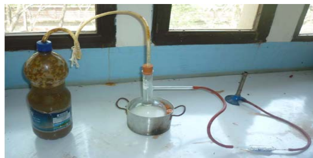
Figure 6: Set up for biogas improvement technique.
