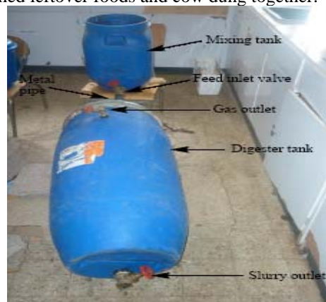
Figure 3: Pilot scale digester fixed with mixing tank.
