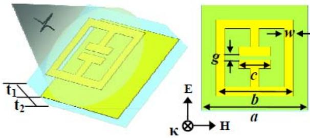
Figure 3: Metamaterial absorber. Figure adapted from [15]
