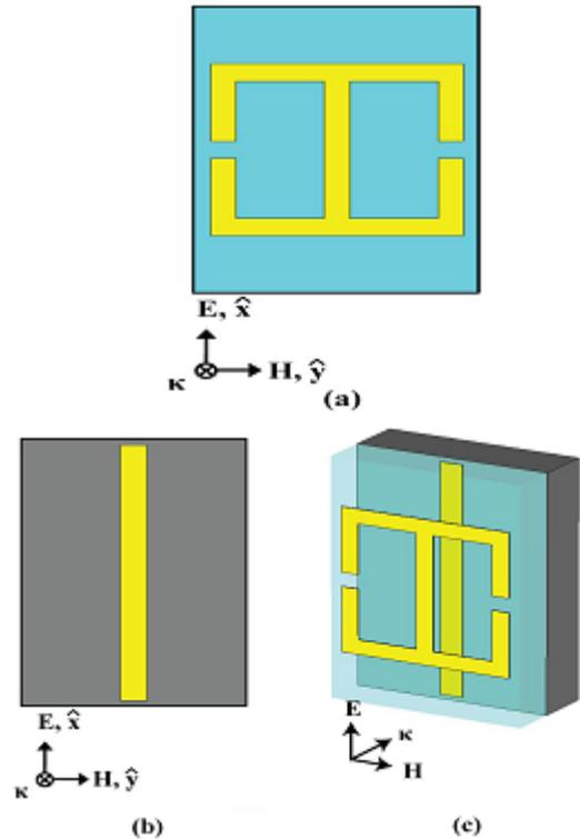
Figure 5: (a) Electric resonator (b) Cut wire (c) Single unit cell showing the direction of propagation of incident EM wave. Figure adapted [16]
