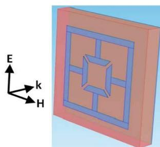
Figure 7: Unit cell of THz absorber. Figure adapted from [17]
