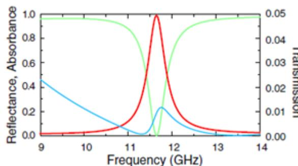
**Figure 2:** Simulated metamaterial perfect absorber. Reflectance (green color), transmission (blue color) and absorption (red color). Figure adapted from Physics Review letters [14]
