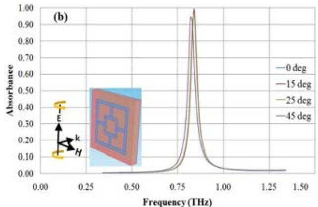
Figure 9: Absorption spectra for incident angles rotation about (a) MF (b) EF. Figure adapted from [17]
