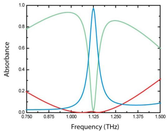
(d) The absorption (blue) yields a value of 98% at 1.12 THz, reflection (green) and transmission (red) both at normal incidence. Figure adapted from [16]
