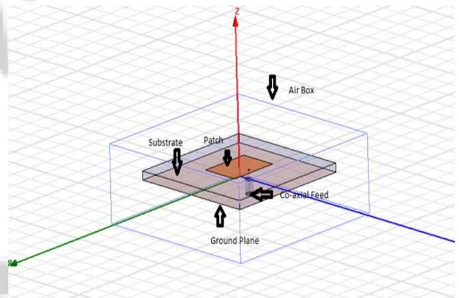
**Figure 2:** The microstrip patch antenna design in HFSS
