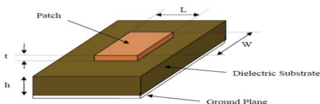
**Figure 1:** Basic structure of Rectangular Micro strip Antenna.
