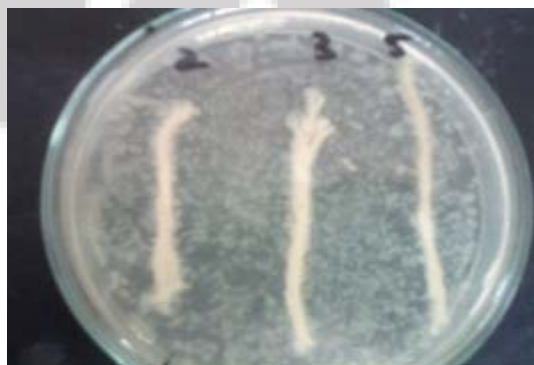
Figure 2: Antimicrobial test of chitosan (2g to 6g) and silver (1ml) coated cotton yarn
