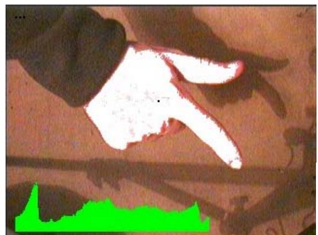
Figure 6.1: Images showing the histogram for two different gestures. The two histograms are sufficiently different to permit differentiation
