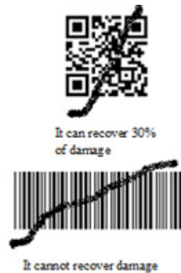
Figure 1(c): The data recovery for damaged code in one and two dimensional codes [4]
