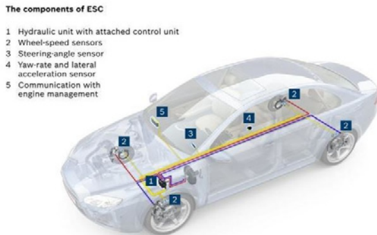
Figure 2.2: Four wheeler (Car) fitted with ESC
