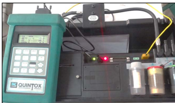
Figure 9: Flue Gas Analyzer
