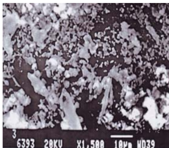
Figure 3: Scanning Electron micrograph of kieselguhr particles
