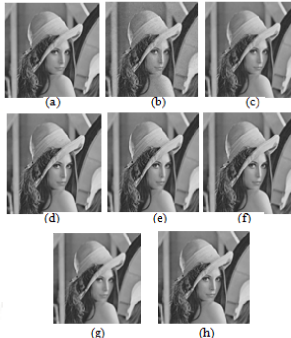
Figure 4: (a) Original Image (b) Noisy Image (c) 3x3 Median Filter (d) 3x3 IQR Filter (e) 5x5 Median Filter (f) 5x5 IQR Filter (g) 7x7 Median Filter (h) 7x7 IQR Filter
