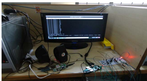
Figure 7: Dissolved oxygen sensor, GSM, Speakers are interfaced to raspberry pi
