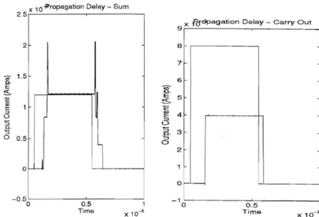
Figure 6: SPICE Model Propagation Delay for Sum and Carry Out
