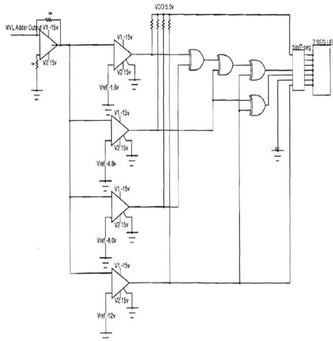
Figure 4: Testbench Output Circuitry
