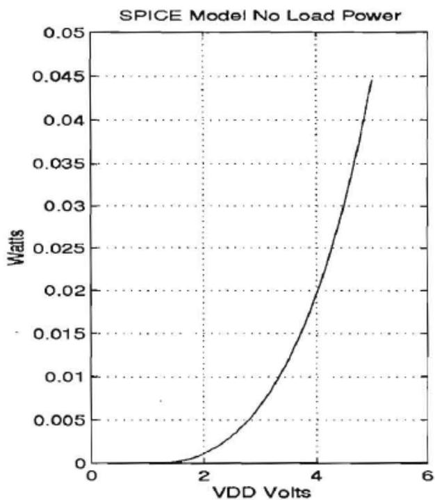
Figure 5: Measured and SPICE Simulation of No Load Static Power Consumption
