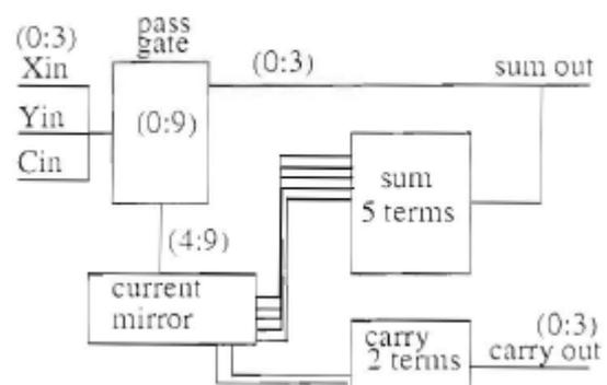
Figure 1: Block Diagram of New 'Modulo 4 adder
