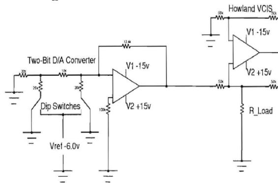
Figure 3: Testbench Input Circuitry
