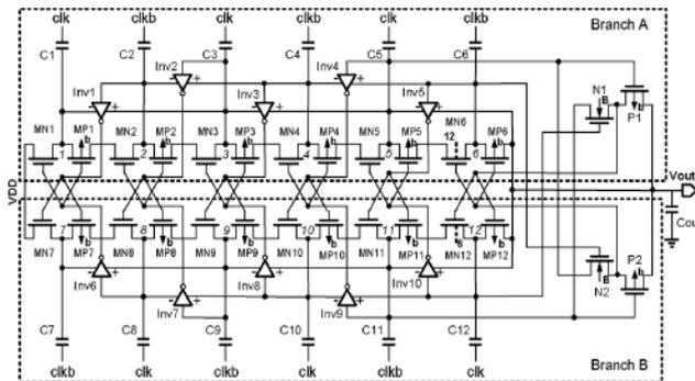
Figure 2: Proposed Charge pump with inverter stages
