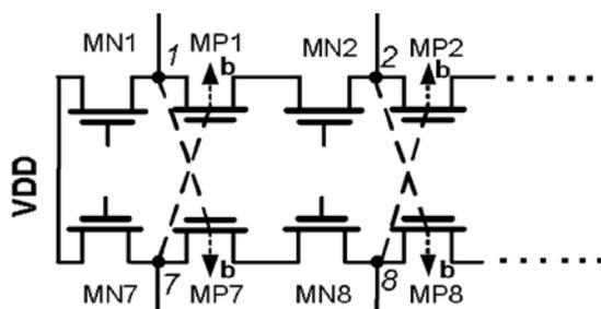
Figure 3: Body biasing from the node of operation
