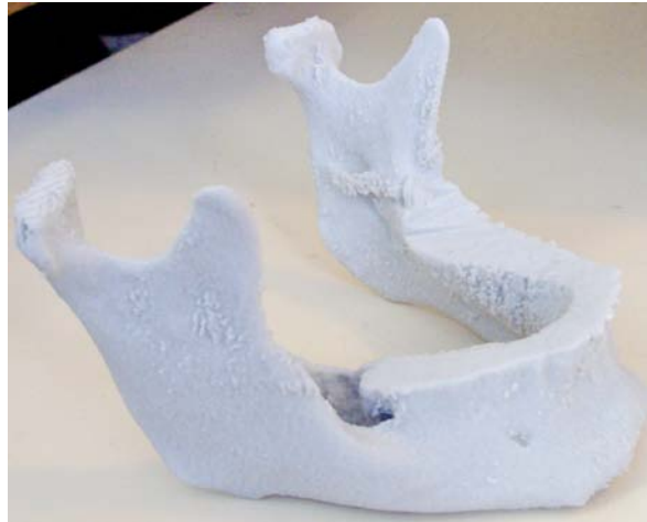
Figure 2: The mandible prototype used for preparing of the titanium plate. The shape of the mandible and the bone defect of the tumor are well visible.
