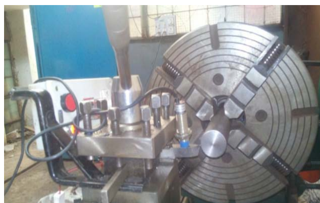
Figure 3: Actual experimental set up to measure normal force
