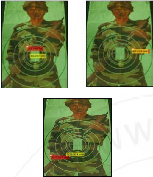
Figure 2: Frame showing 1 st , 2 nd , 3 rd , 4 th and 5 th fire point with distance from Centre
