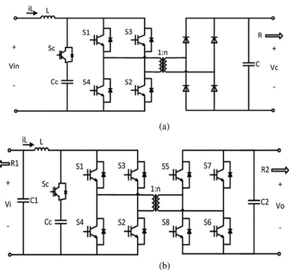
**Figure 2:** Topological circuit of the converters under study: (a) boost and (b) bidirectional.
