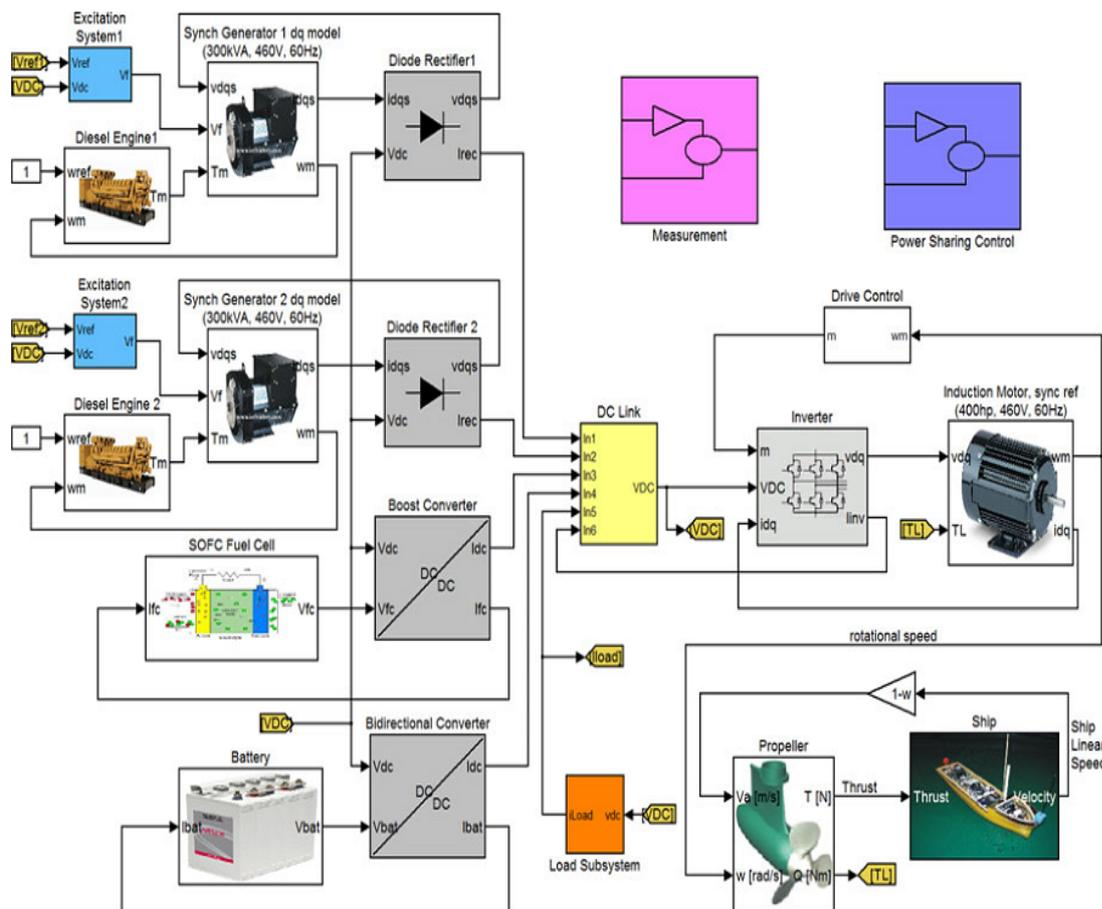
**Figure 4:** Overview of the ship dc hybrid power system implemented in MATLAB/Simulink
