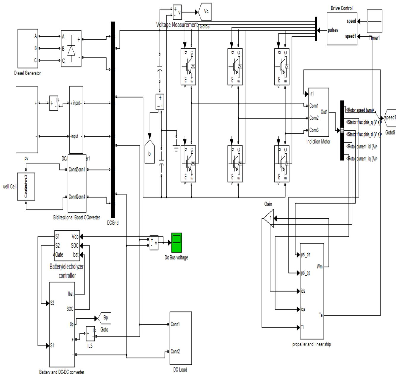
Figure 5: Simulation Model Ship DC Hybrid Power System
