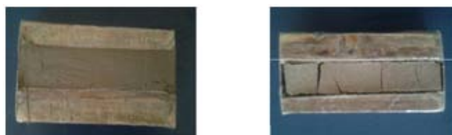
Figure 7: Shrinkage of 50% BC soil + 50% Brick dust
