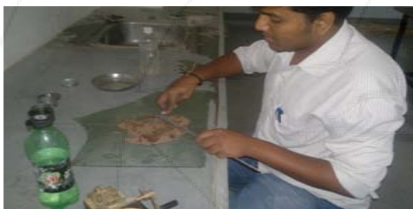
Figure 2: Determination of Liquid limit & Plastic limit
