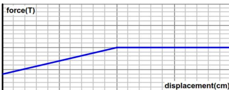
Figure 5: Constitutive law of the spring replacing the non-active subgrade.
