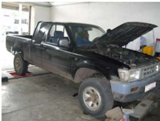
Figure 1: Twin roller chassis dynamometer
