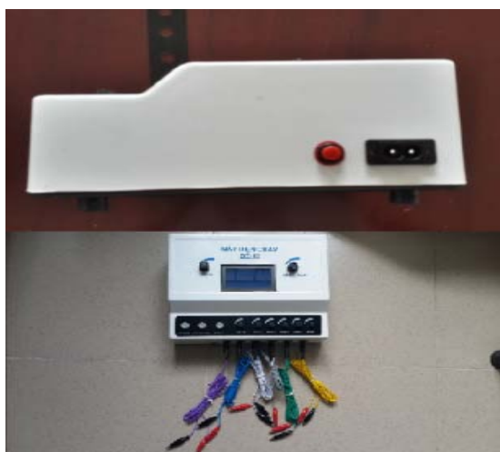
Figure 5: DC-12 power and outputs
