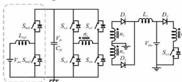
Figure 7: Proposed integrated full-bridge-forward dc-dc converter including a bidirectional converter
