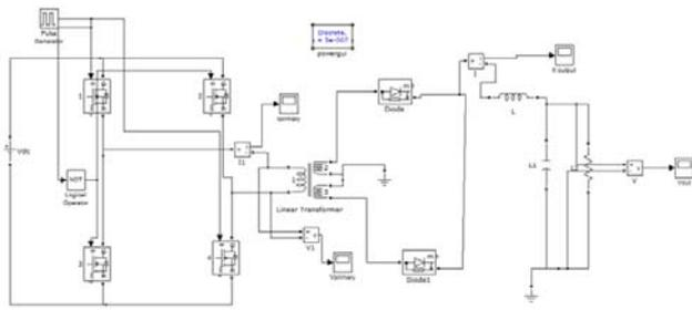
Figure 12: The Matlab/Simulink model of full-bridge Converter
