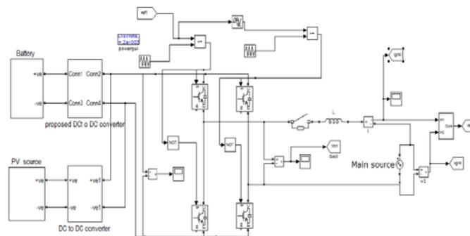
**Fig. 16.** The Matlab/Simulink model of integration of storage device using proposed converter in residential microgrid system.
