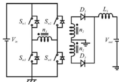
Figure 5: Full-bridge converter
