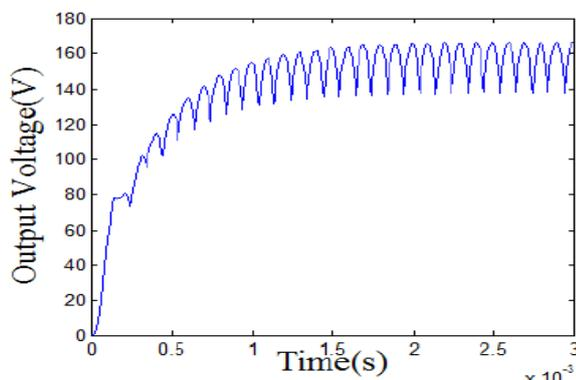
Figure 4: Output voltage of DAB converter
