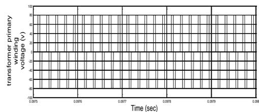
Figure 13.1: Transformer primary winding voltage
