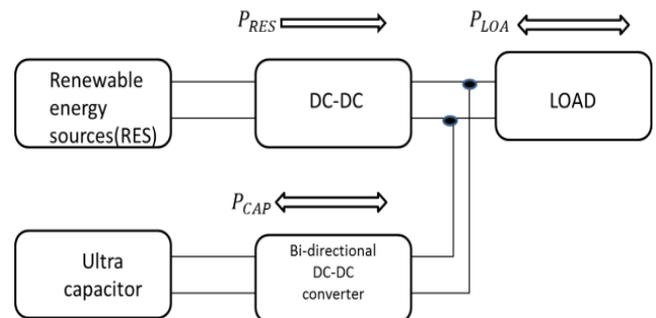
**Figure 2:** Block diagram of energy storage augmented renewable source system
