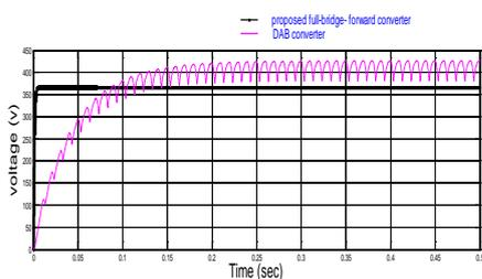
**Figure 15:** Comparison of proposed converter with dual active bridge converter (DAB).
