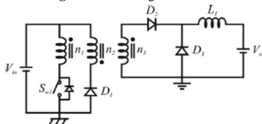
Figure 6: Forward converter
