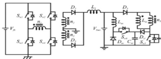
Figure 9: Proposed converter with regenerative active clamping circuit
