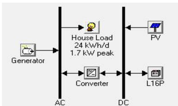
**Figure 1:** Residential microgrid system under study
