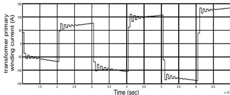
Figure 1.2.1: Transformer primary winding current
