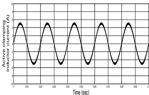
**Figure 14.2:** Active clamping circuit inductor current.
