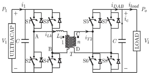
Figure 3: Dual active bridge(DAB) converter.
