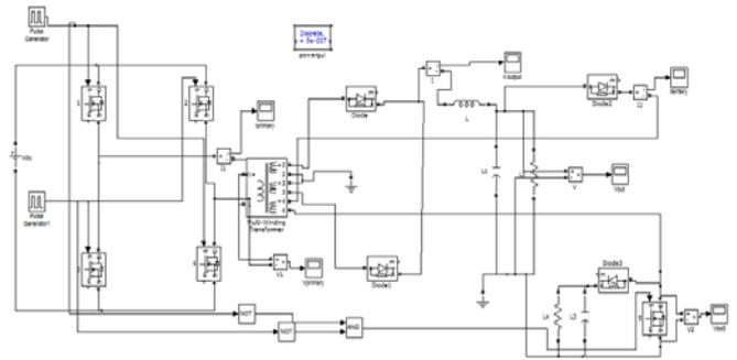
Figure 13: The Matlab/Simulink model of full-bridge forward converter with dissipative passive clamping circuit.
