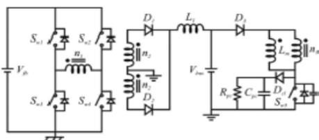
Figure 8: Integrated full-bridge-forward converter including dissipative passive clamping circuit
