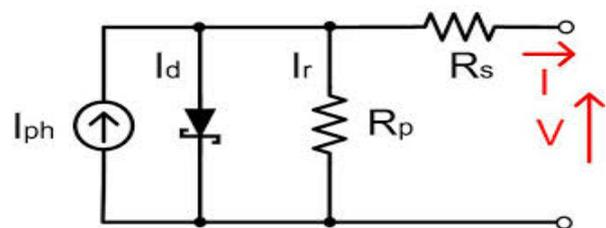
Figure 10: Equivalent circuit of PV cell.
