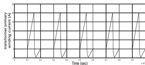
Figure 13.2: Transformer primary winding current
