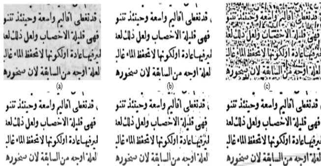
Figure 4: Binarization results of an Arabic historical document image: (a) Original image, (b) Otsu's, (c) Niblack's, (d) Sauvola's, (e) NICK and (f) Proposed method.
