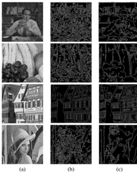
Figure 11: Comparison of the edge maps of noisy images by using the original Canny edge detector and the proposed method: (a) images with Gaussian white noise ( \sigma_n = 0.01 ); edge-maps of (b) the original Canny edge detector, and (c) the proposed algorithm with a non-overlapping block size of 64 \times 64 , using a 9 \times 9 gradient mask to noise than the original frame-based Canny.
