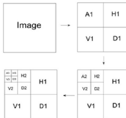
Figure 3: DWT multilevel decomposition of an image
