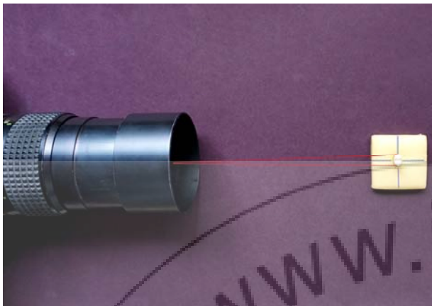
Figure 1: A custom-made device was constructed to hold the teeth in the same position
