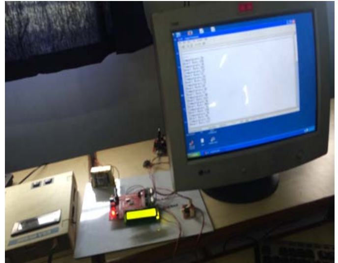
Figure 4: Patient Health Monitoring By ZIGBEE Communication
