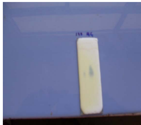
Figure 1: The chromatograms of the elute having similar spots as the marker methyl gallate
